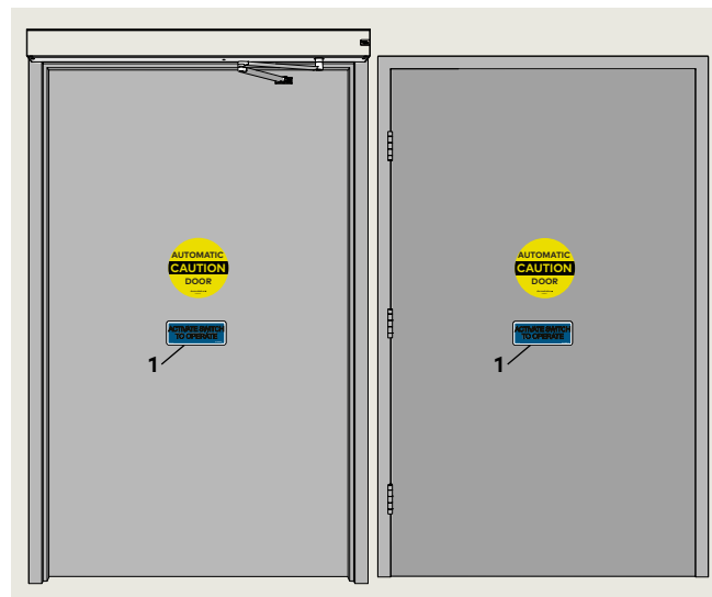
Fig. 11.2.1 Knowing act device initiation of door operation
